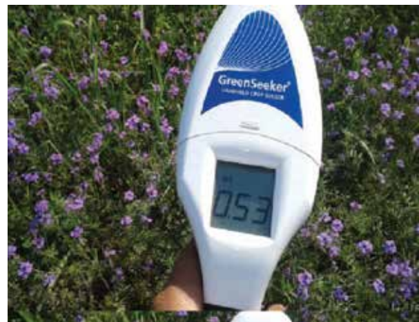
Fig. 2b. A handheld NDVI sensor to assess crop health.
