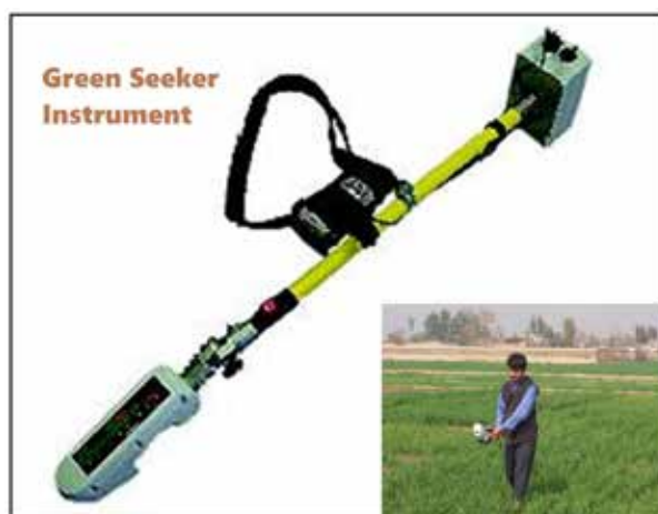
Fig. 2a. Handheld Green Seeker instrument for NDVI measurement.
