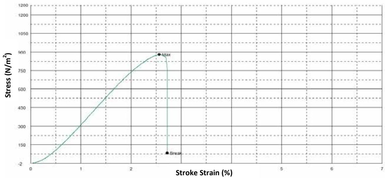
Fig. 6 (b). Tensile testing graph for  $Ti_{91}Al_5V_4$ .
