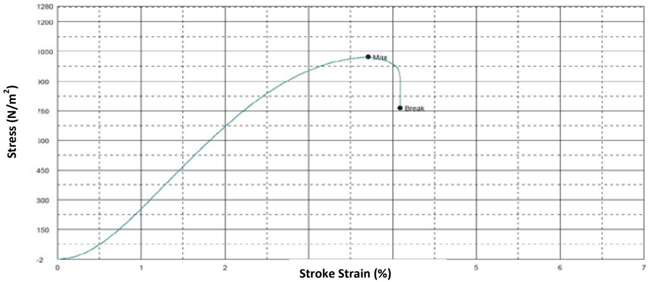
Fig. 7(b). Tensile testing graph for  $Ti_{90.5}Al_{5.5}V_4$ .
