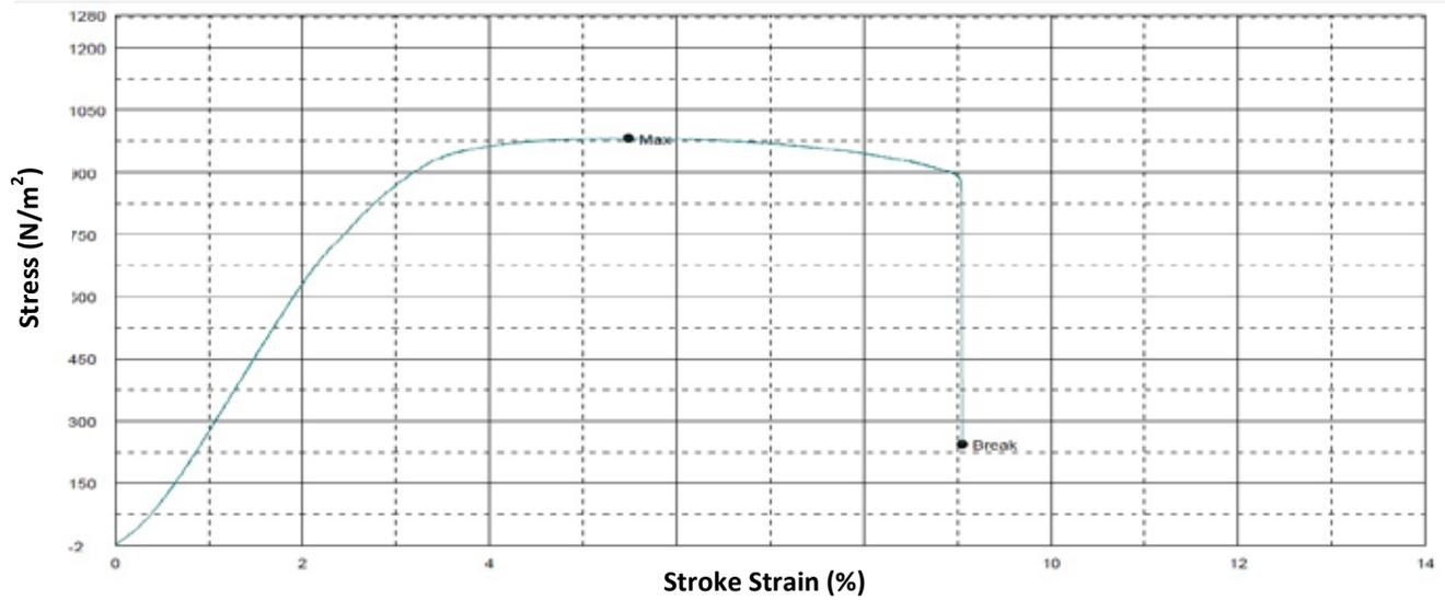
Fig. 8 (a). Tensile testing graph for  $Ti_{89.5}Al_{6.5}V_4$ .
