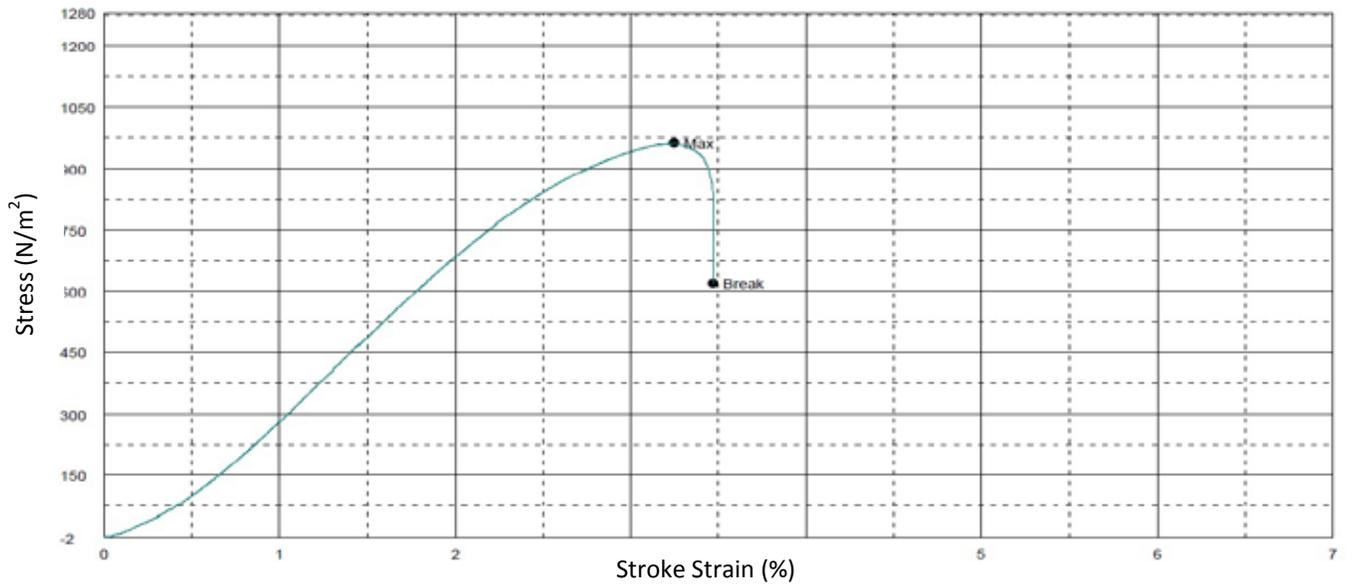
Fig. 7(a). Tensile testing graph for  $Ti_{90.5}Al_{5.5}V_4$ .
