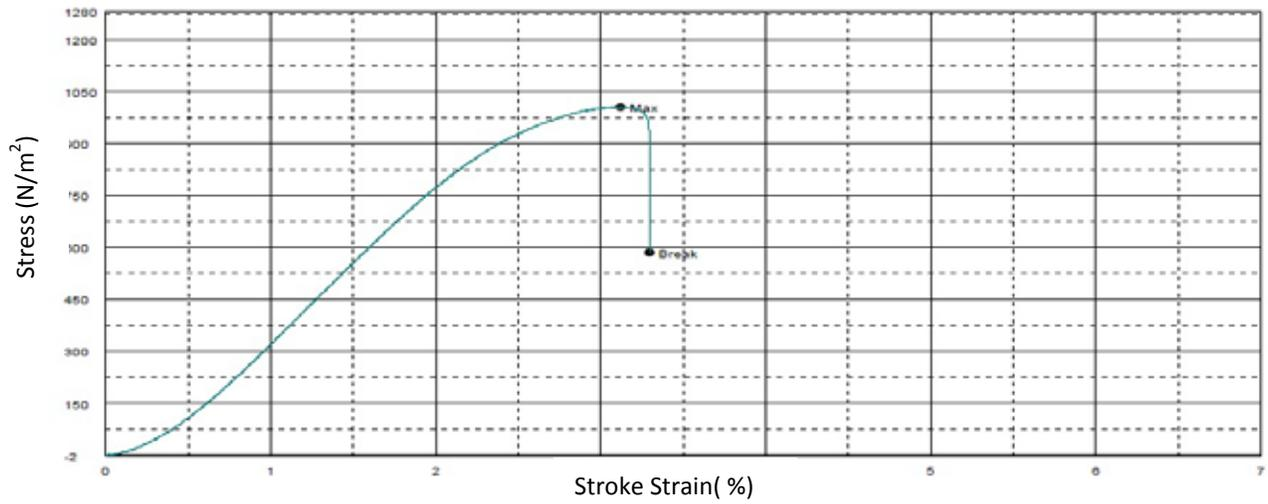
Fig. 6 (a). Tensile testing graph for  $Ti_{91}Al_5V_4$ .
