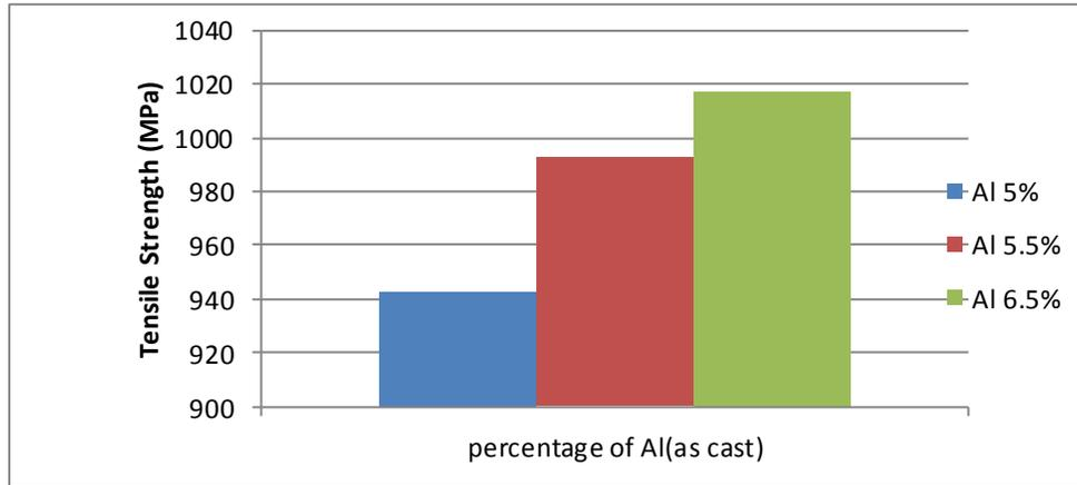
Fig. 9. Comparison of tensile strength in MPa.
