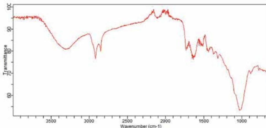
Fig. 2. Spectrum of banana peel treated with sulfuric acid.
