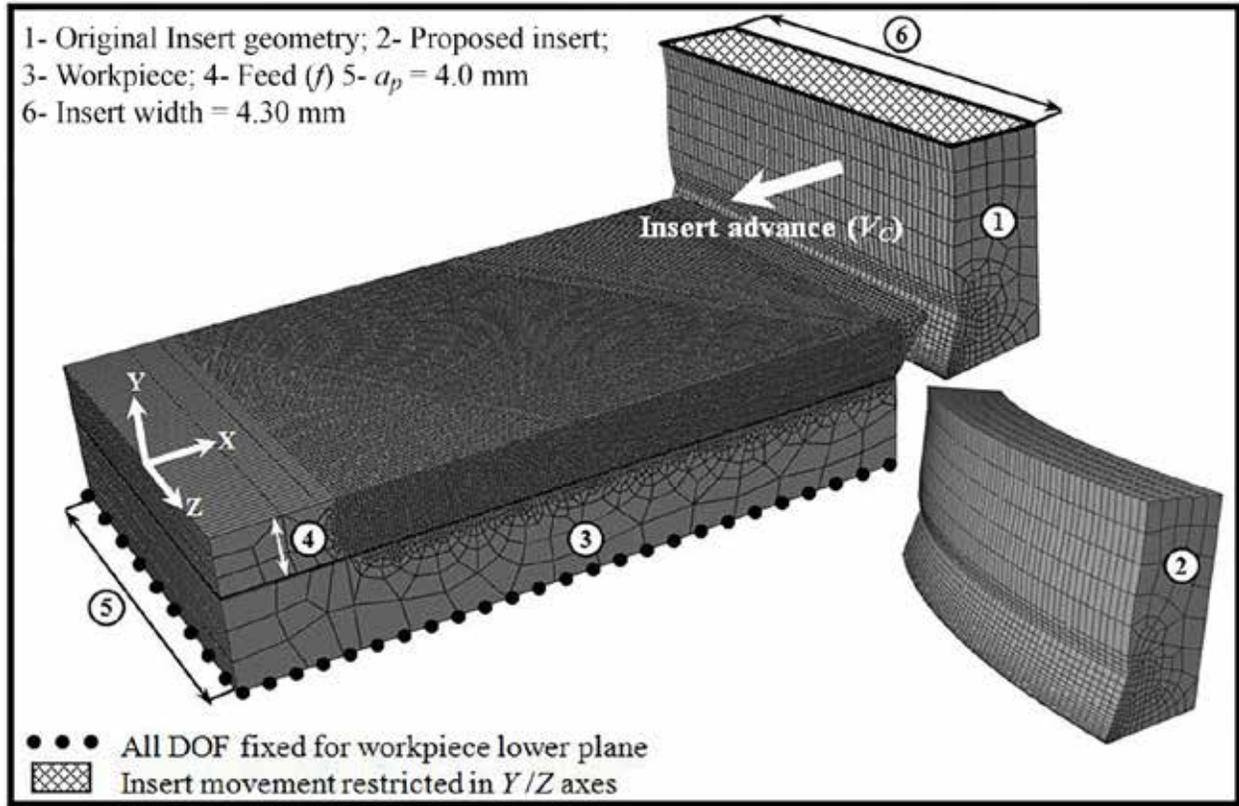
Fig. 1. Three-dimensional work-piece and turning inserts models.
