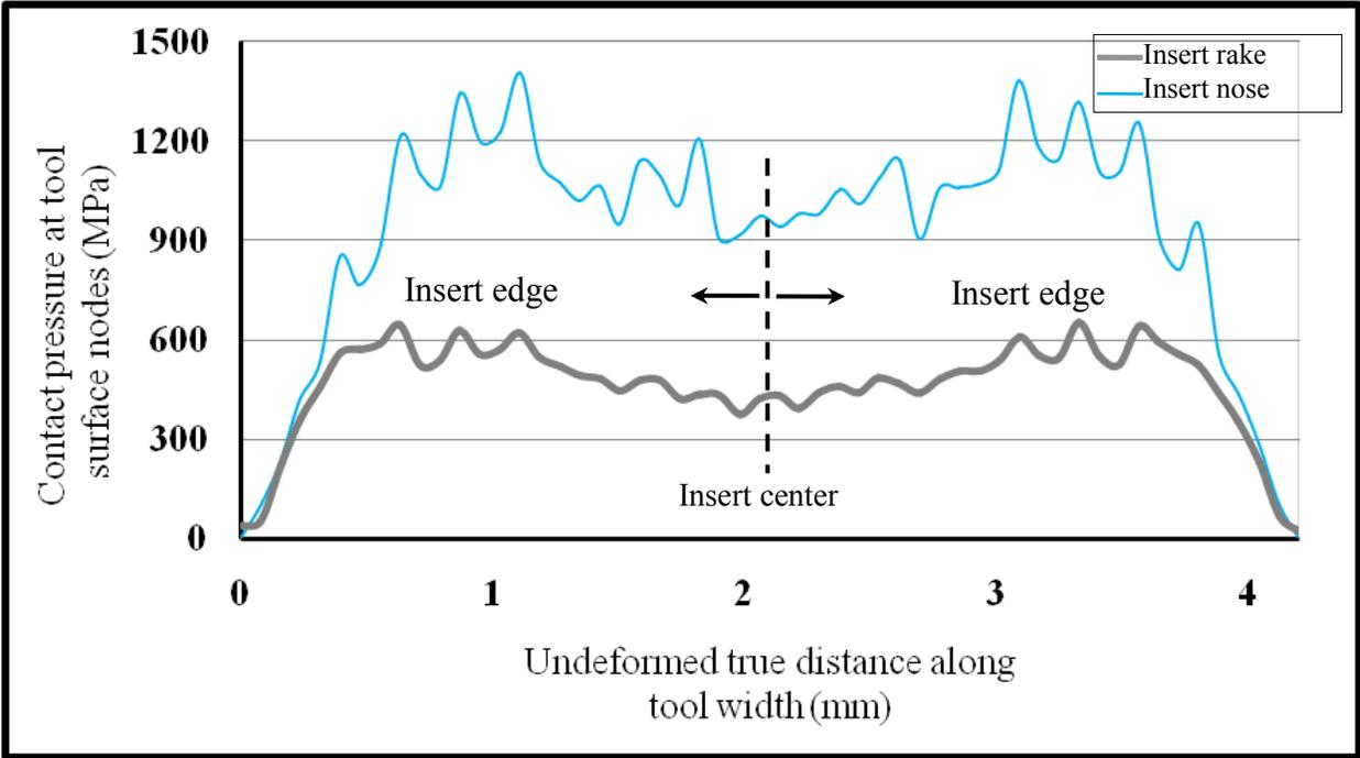
Fig. 4. Profiles of contact pressure at various contact sections of cutting insert for  $V_c = 800$  m/min,  $f = 0.5$  mm/rev,  $a_p = 4$  mm.
