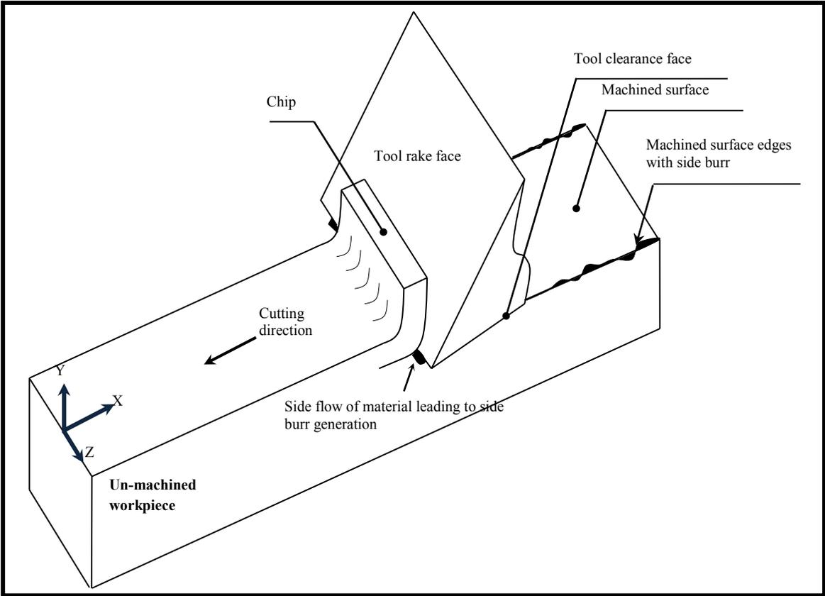
Fig. 3. Side burr formation in turning operation.
