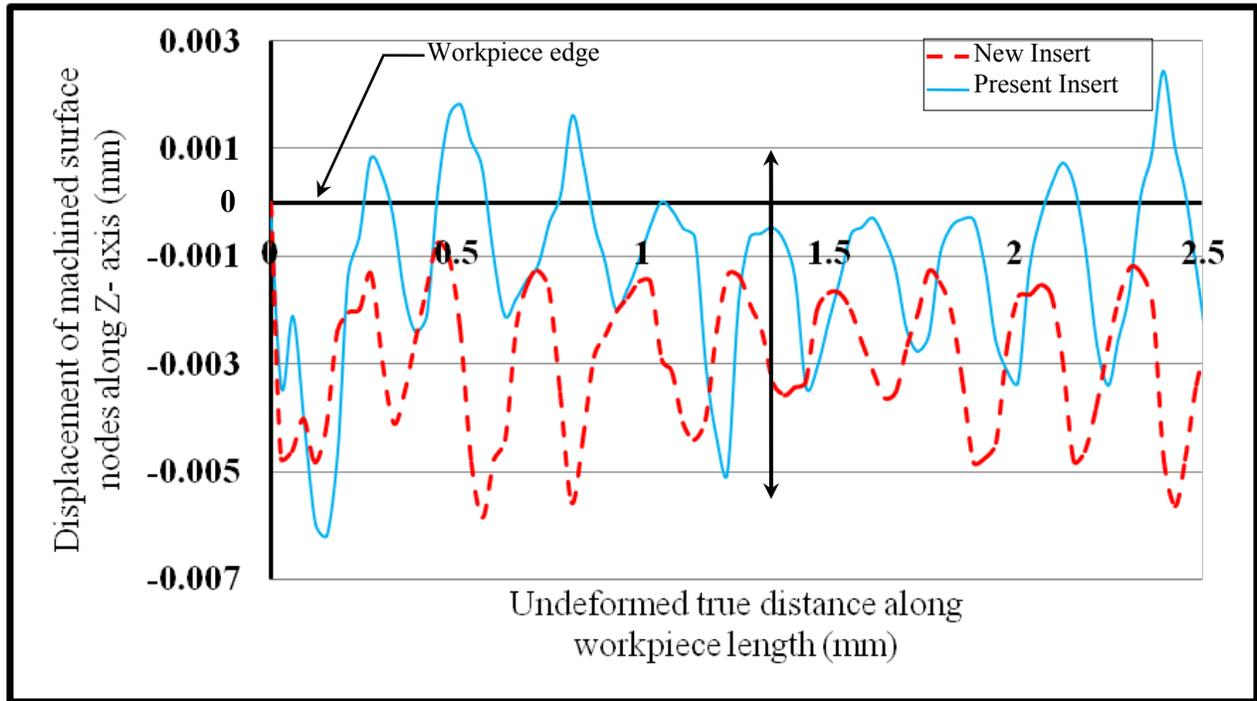
Fig. 5. Quantitative prediction of side burr for  $V_C = 800$  m/min,  $f = 0.5$  mm/rev,  $a_p = 4$  mm.
