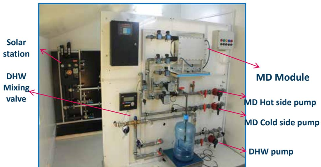
**Fig. 5.** MD system with solar station.
