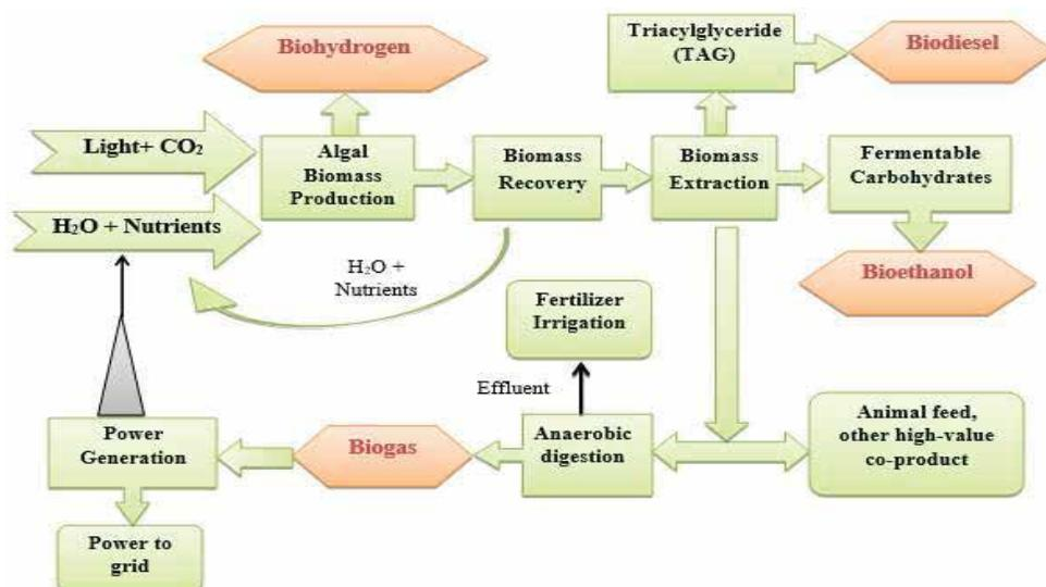
**Fig. 3.** A conceptual model for integrated microalgal biomass and biofuel production [5].
