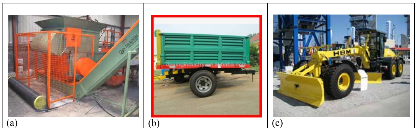
Fig. 10. Proposed steps for polythene/polyester fibers stabilization at construction site: (a) Fibers shredding; (b) Fibers spreading; (c) Fibers mixing with soils (Photos courtesy of Google Images, http://www.google.com ).
