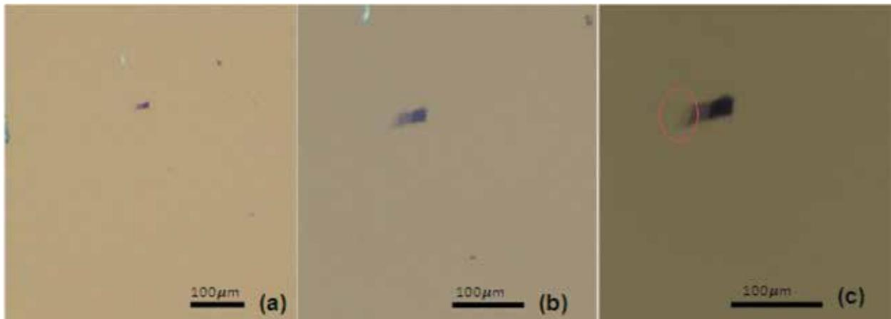
**Fig. 8.** Optical image of fourth flake over 90nm Si/SiO<sub>2</sub> substrate at: (a) 20x; (b) 50x; (c) 100x.
