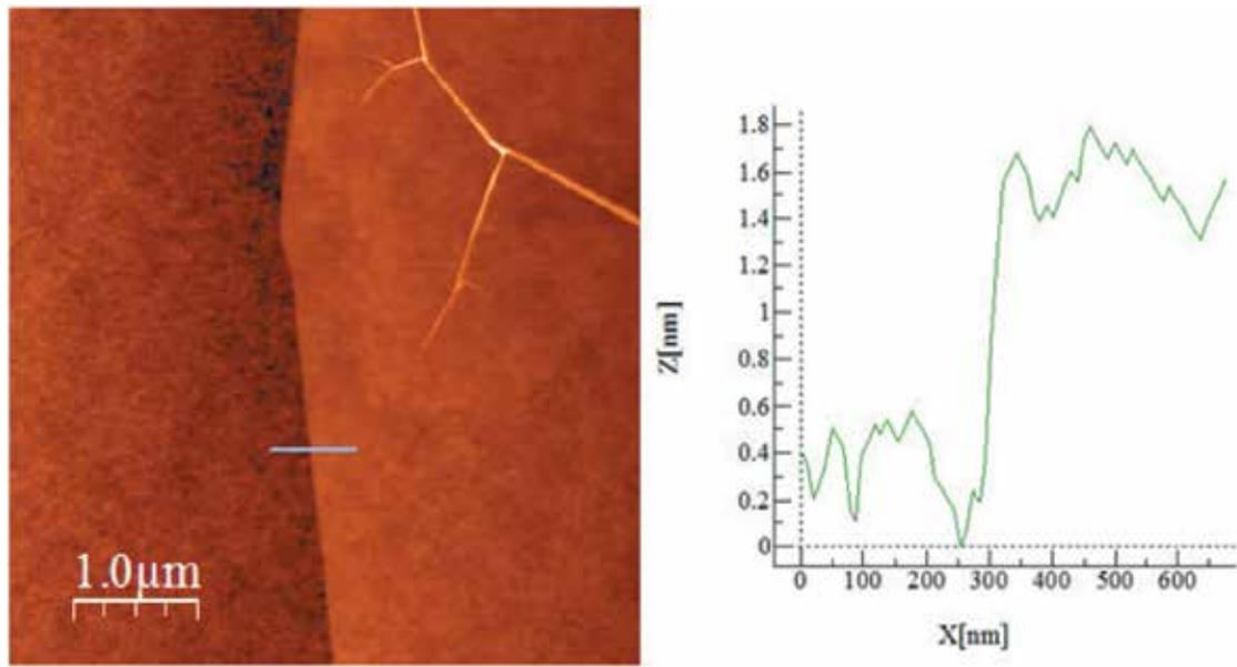
Fig. 19. Step height  $\sim 1.0$ nm (3 layers).
