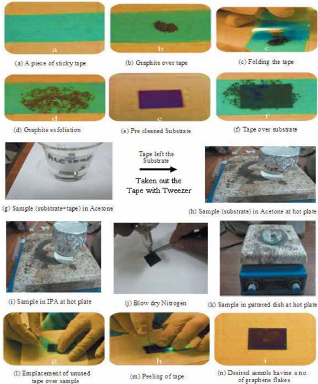
**Fig. 3.** Schematic of micromechanical cleavage method to fabricate graphene on Si/SiO<sub>2</sub> substrate.
