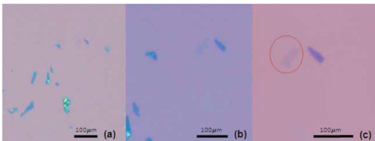
**Fig. 11.** Optical image of second flake over 300nm Si/SiO<sub>2</sub> substrate at: (a) 20x; (b) 50x; (c) 100x.
