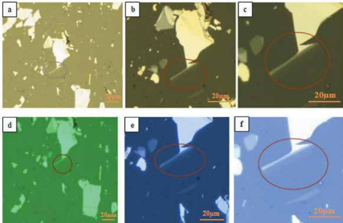
**Fig. 15.** Optical images of graphene flake on PMMA substrate: (a) at 20x using white light; (b) at 50x using white light; (c) at 100x using white light; (d) at 20x with green filter; (e) at 50x with blue filter; (f) at 100x with blue filter.
