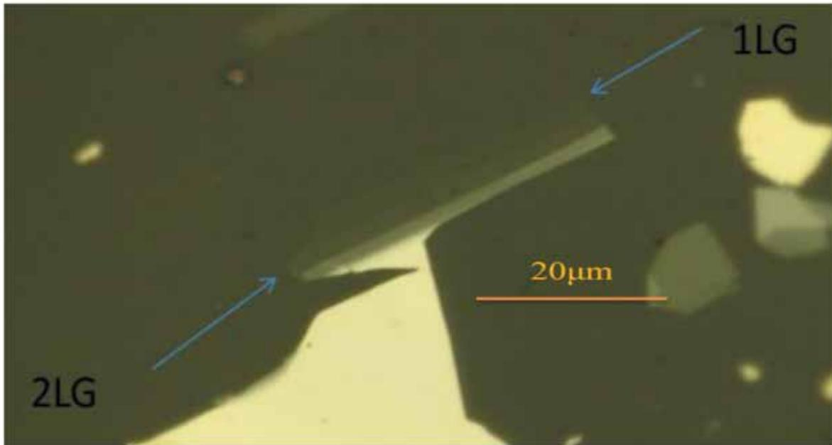
**Fig. 13.** Optical image for single (1LG), bi-layer (2LG) and few-layer graphene on PMMA substrate at 100x.
