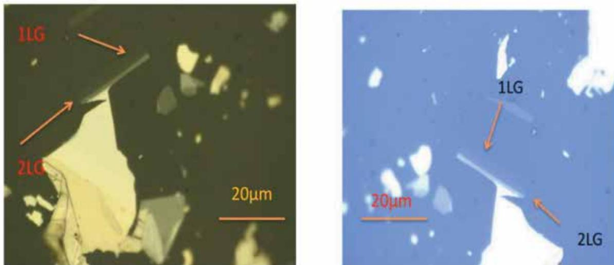
**Fig. 14.** Improvement in the optical contrast of graphene flakes using optical filter.
