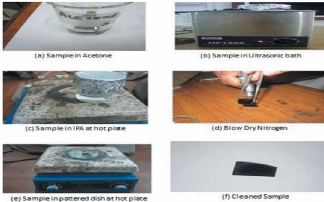
Fig. 1. Standard cleaning method used for Si/SiO<sub>2</sub> substrate.
