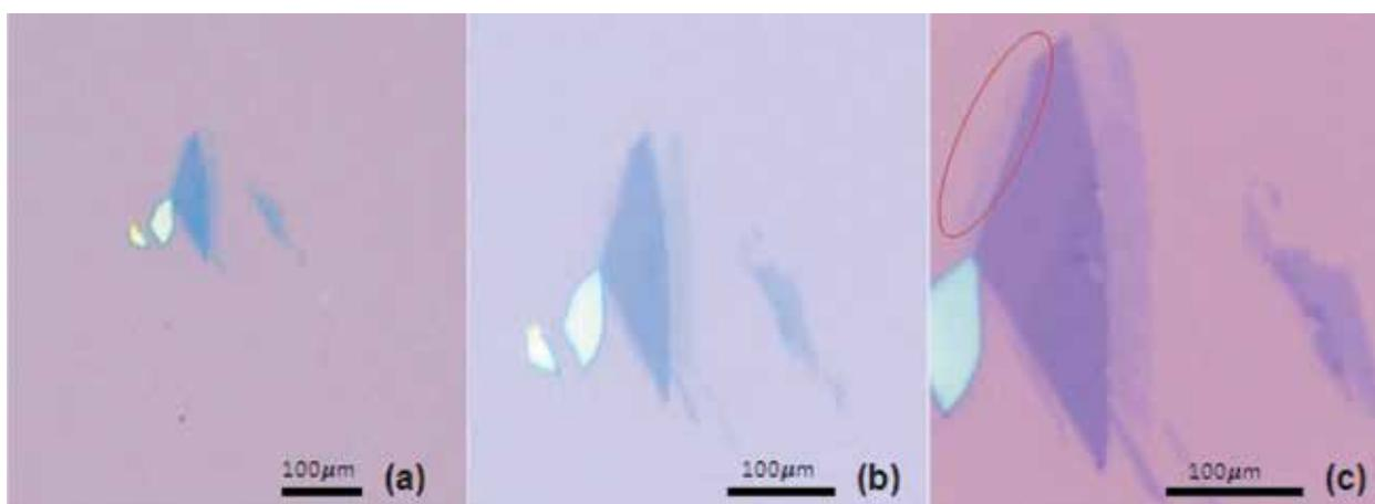
**Fig. 12.** Optical image of third flake over 300nm Si/SiO<sub>2</sub> substrate at: (a) 20x; (b) 50x; (c) 100x.
