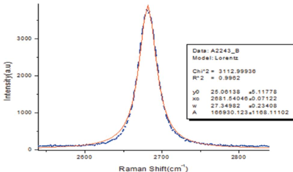
Fig. 21. Determination of width of 2D band by Lorentz fitting.
