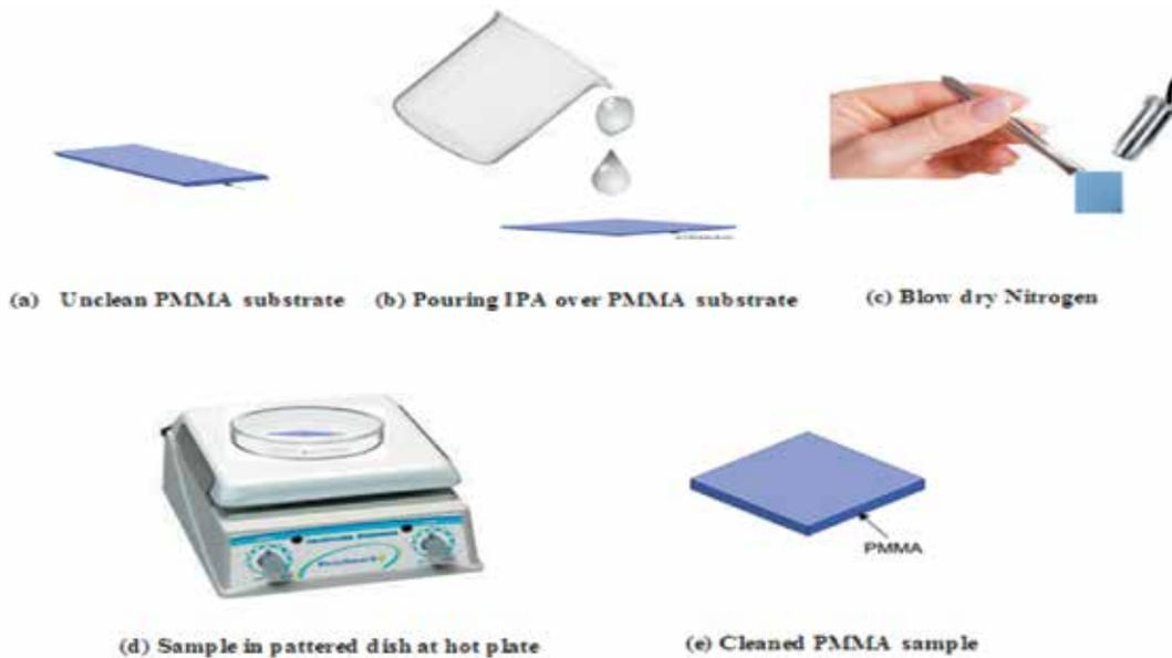
Fig. 2. Schematic of standard cleaning method for PMMA substrate.
