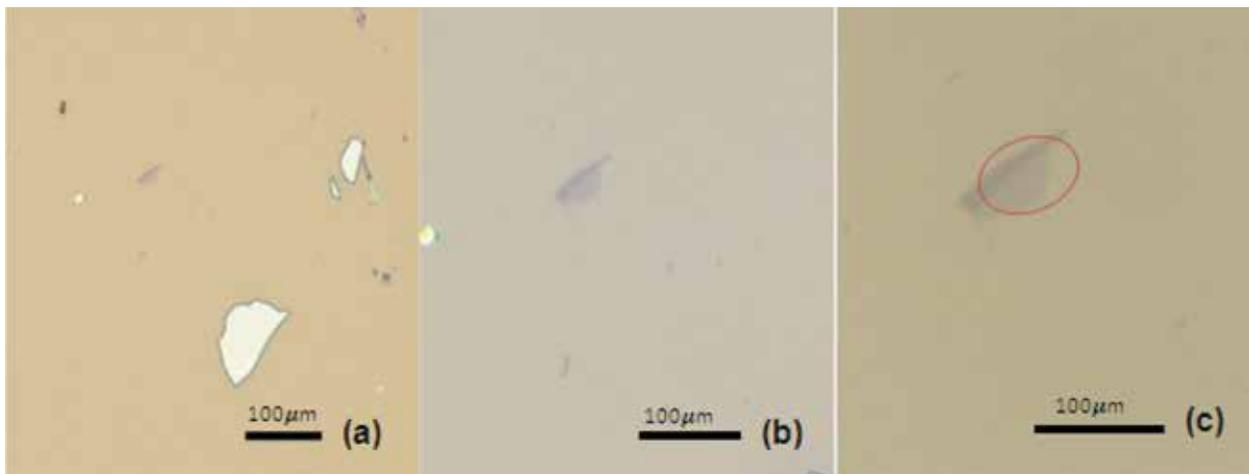
**Fig. 9.** Optical image of fifth flake over 90nm Si/SiO<sub>2</sub> substrate at: (a) 20x; (b) 50x; (c) 100x.
