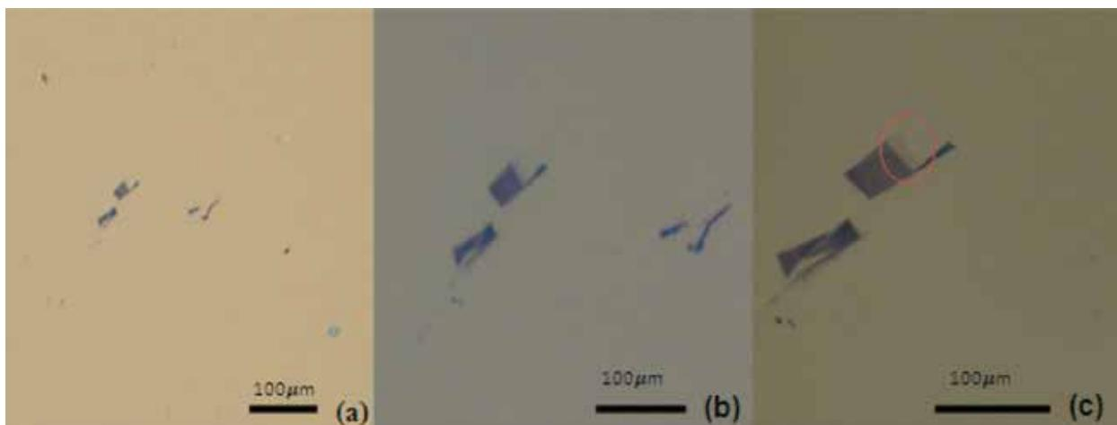
**Fig. 5.** Optical image of first flake over 90nm Si/SiO<sub>2</sub> substrate at: (a) 20x; (b) 50x; (c) 100x.
