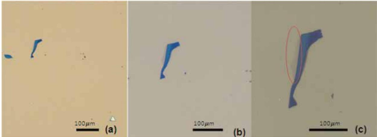
**Fig. 7.** Optical image of third flake over 90nm Si/SiO<sub>2</sub> substrate at (a) 20x (b) 50x (c) 100x.
