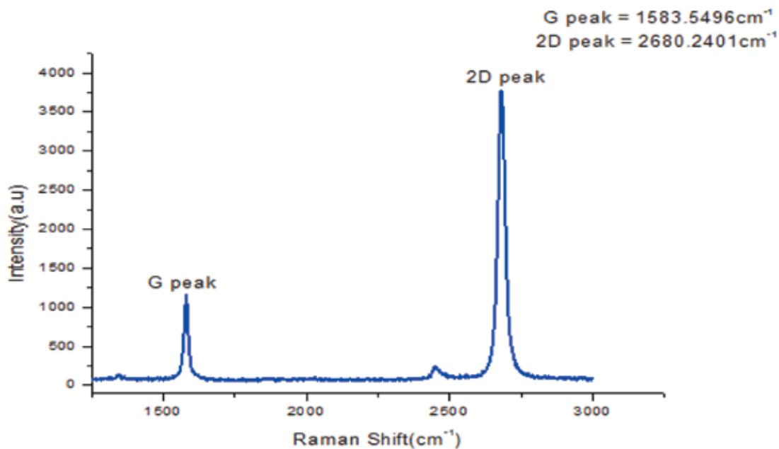
Fig. 20. Raman spectra of single layer graphene on Si/SiO<sub>2</sub> substrate.
