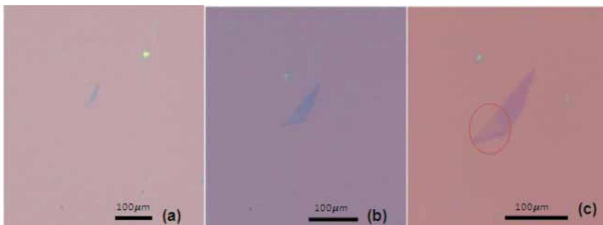
**Fig. 10.** Optical image of first flake over 300nm Si/SiO<sub>2</sub> substrate at: (a) 20x; (b) 50x; (c) 100x.
