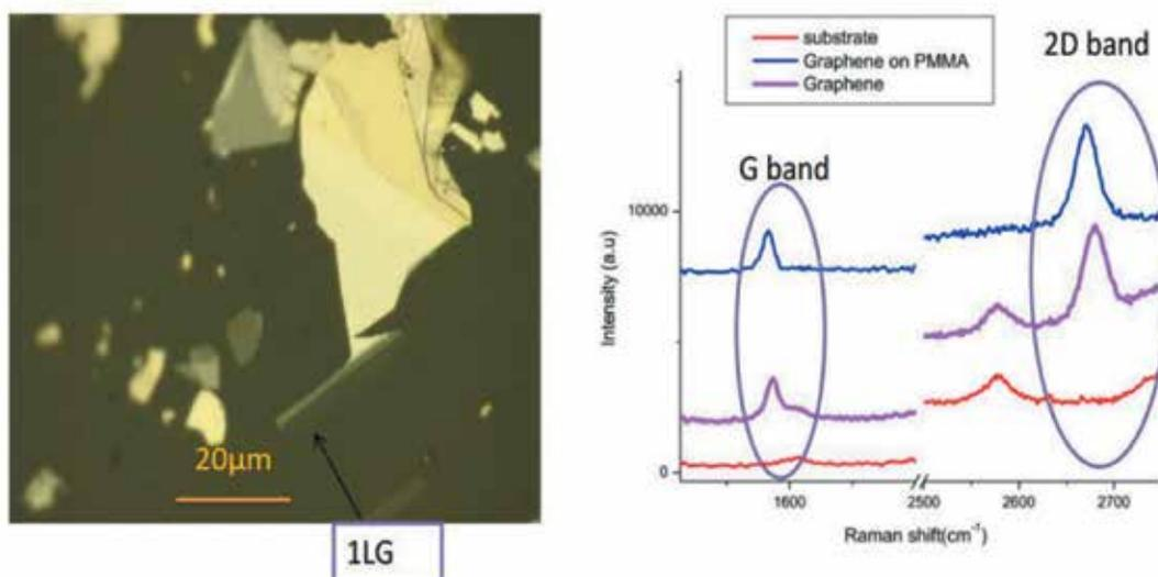
Fig. 22. Raman spectra of monolayer graphene (1LG) over PMMA substrate.
