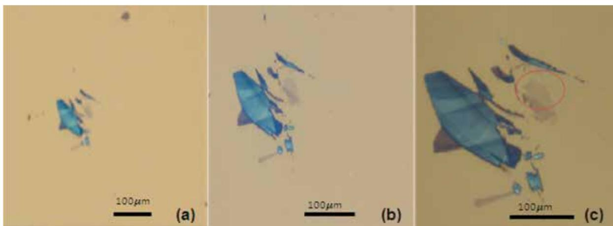
**Fig. 6.** Optical image of second flake over 90nm Si/SiO<sub>2</sub> substrate at: (a) 20x; (b) 50x; (c) 100x.
