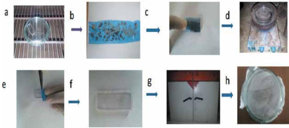
**Fig. 4.** Schematic for the fabrication of graphene on PMMA substrate.
