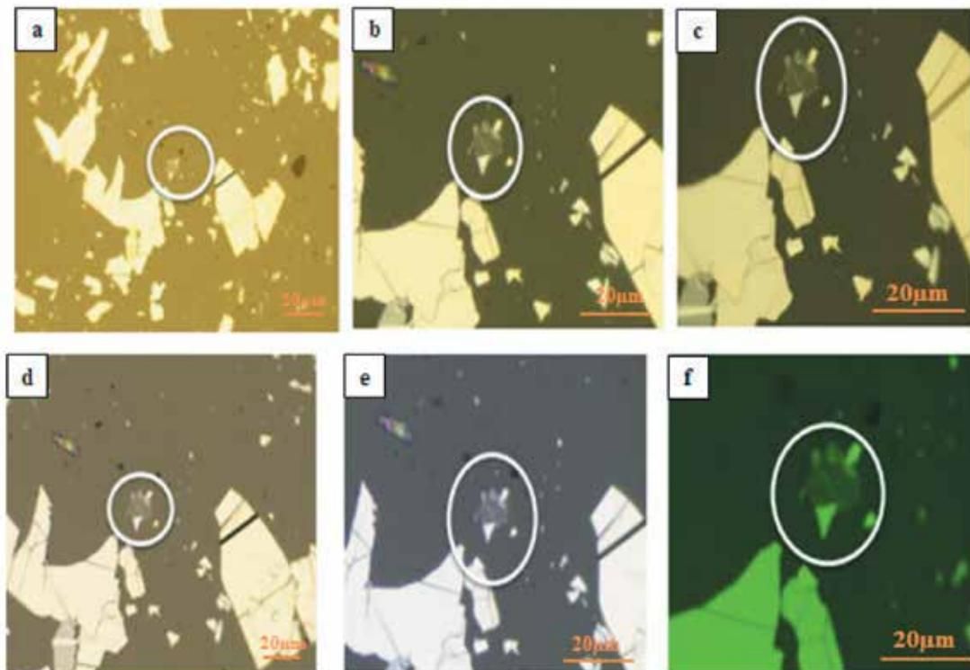
**Fig. 16.** Optical images of graphene flake on PMMA substrate: (a) at 20x using white light; (b) at 50x using white light; (c) at 100x using white light; (d) at 20x with LB145 filter; (e) at 50x with LB145 filter; (f) at 100x with GB530 filter.
