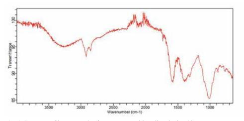
Fig. 4. Spectrum of banana peels after treatment with sodium hydroxide.
