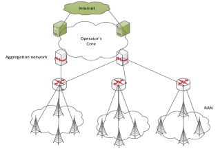
**Fig. 1.** Centralized Mobility Management Architecture
