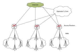
**Fig. 2.** Distributed Mobility Management Architecture/Flat Architecture
