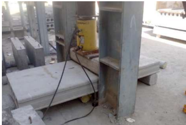
Fig. 3. Testing arrangement for slabs in flexural loading
