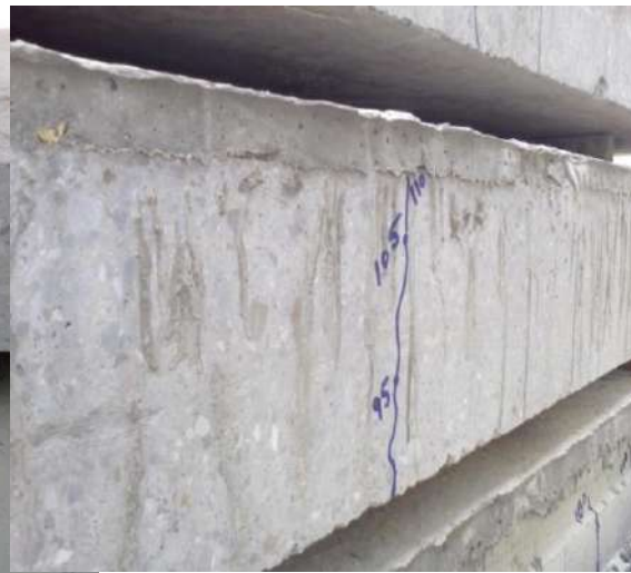
(b) Crack patterns of 200mm depth slab with 32mm topping
