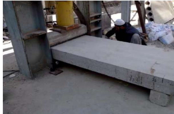
Fig. 4. Testing arrangement for slabs in shear loading
