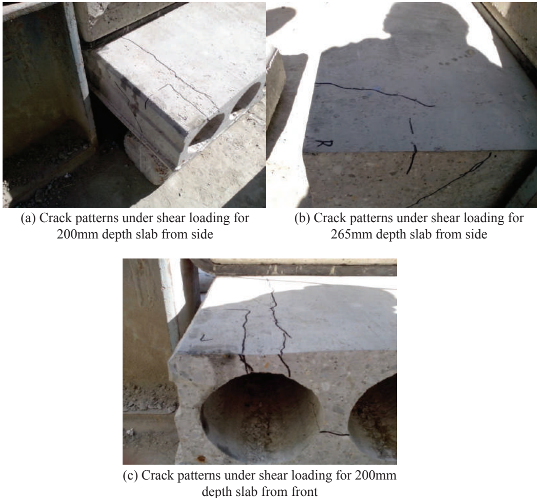
Fig. 12. Crack pattern under shear loading
