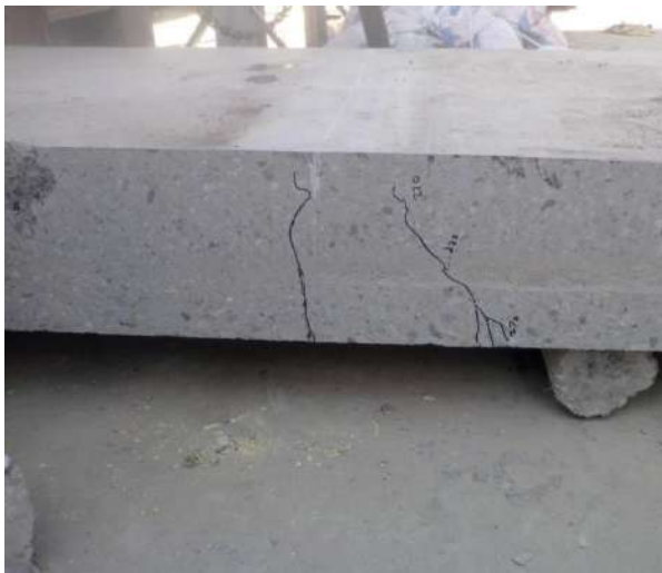
(a) Crack patterns of 265mm depth slab
