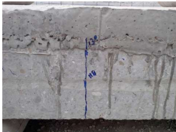
(c) Crack patterns of 200mm depth slab with 65mm topping on top
