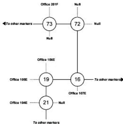
Fig. 3. Final floor graph of the indoor paths of the building after augmentation
