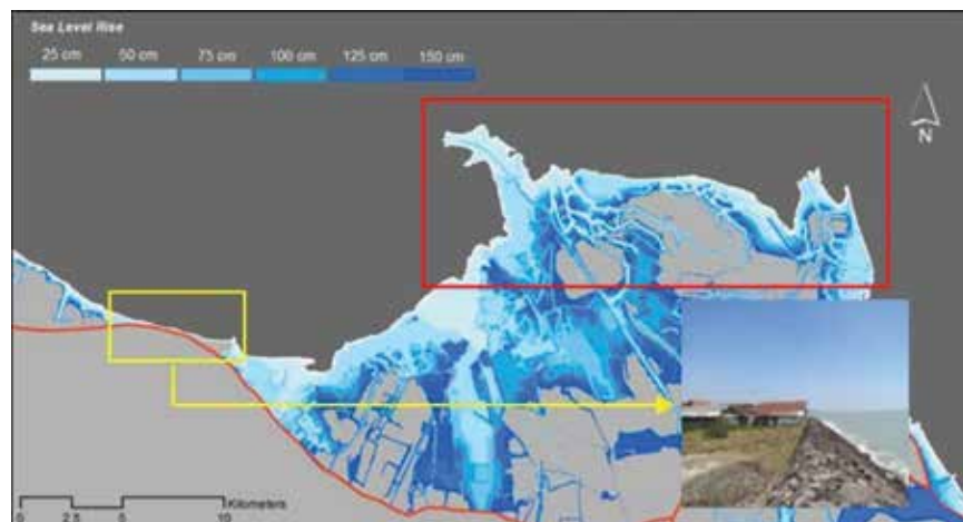
Fig. 6. Coastal inundation map of Indramayu using tidal flood modeling based on sea level rise scenarios (25, 50, 75, 100, 125, and 150) cm
