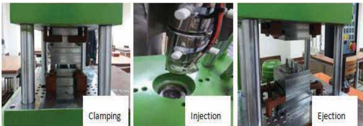
Fig. 2. Different Phases of Injection Molding Process
