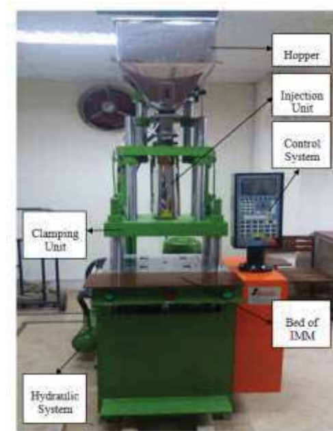
Fig. 1. Vertical plastic injection molding machine
