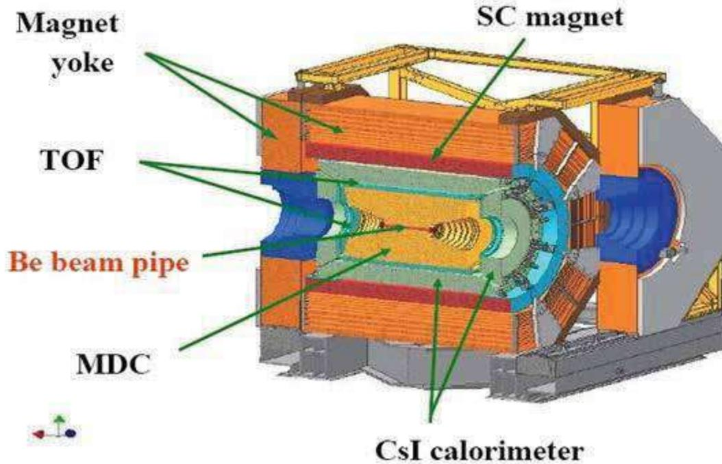
**Fig. 1.** Schematic diagram showing BESIII detector
