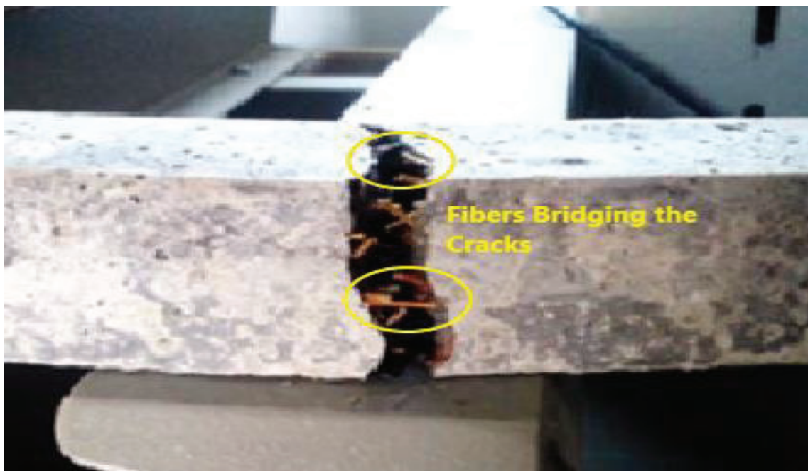
Fig. 8. Pine needles bridging crack in flexural strength test
