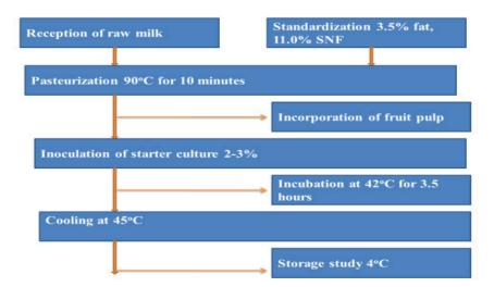
Fig. 1. Schematic diagram of yoghurt supplemented with persimmon
