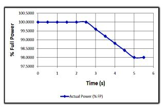
Fig. 20. Reactor Power Ramp-down Transient ACR700 RRS
