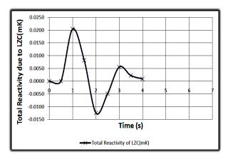
**Fig. 18.** Prediction of Power Error and Reactivity under Small Power Perturbation Maneuvering Transient of ACR700 RRS
