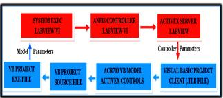
Fig. 9. Integration of LabVIEW and Visual Basic
