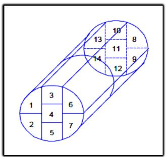
Fig. 3. Configuration of Liquid Zones in ACR700
