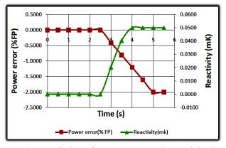
**Fig. 21.** Prediction of Power Error and Reactivity in Power Ramp-down Transient of ACR700 RRS
