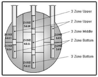
Fig. 4. Physical Visualization of Liquid Zones in ACR700
