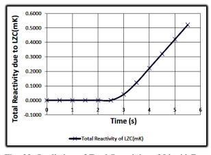
**Fig. 22.** Prediction of Total Reactivity of Liquid Zone Control System in Power Ramp-down Transient of ACR700 RRS
