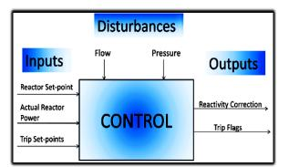
Fig. 7. Overall Control Framework of RRS in ACR700
