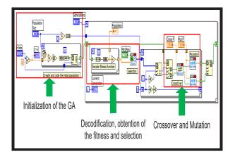
**Fig. 13.** Block Diagram Design of GA Optimization of ACR700 ANFIS RRS Controller in LabVIEW
