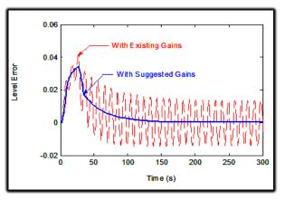
**Fig. 26.** Performance Comparison of Zone Control Compartment Water Level Error under Low Power Transient for ACR700 RRS
