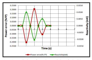
**Fig. 19.** Prediction of Total Reactivity of Liquid Zone Control System under Small Power Perturbation Maneuvering Transient of ACR700 RRS
