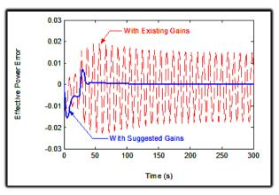
**Fig. 24.** Performance Comparison of Effective Reactor Power Error under Low Power Transient for ACR700 RRS
