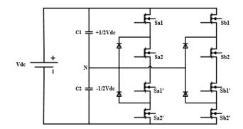
Fig. 11. Full bridge 3L NPC inverter
