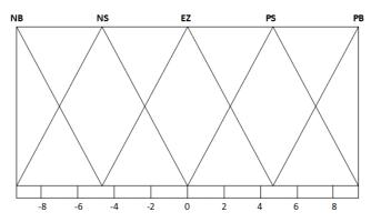
Fig. 4. Input membership function Vpv
