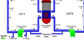
**Fig. 2.** Two loop primary circuit design of PWR in LabVIEW
