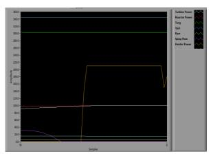
**Fig. 9.** Trends of pressurizer parameters from 100 % to 90 % power transient at  $51^{st}$  sample state.
