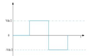
Fig. 10. Output of single phase of NPC inverter
