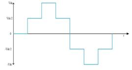
Fig. 12. Line voltage of 3L NPC inverter
