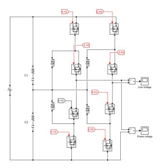
Fig. 19. Simulation of full bridge NPC inverter
