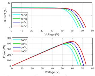
Fig. 2. Temperature effects on solar panels
