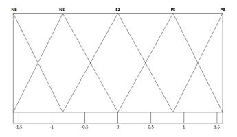
Fig. 5. Input membership function Ipv
