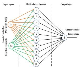
Fig. 2. 3 layered Feed-forward neural network
