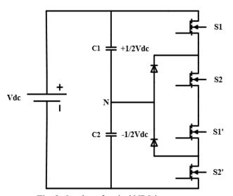
Fig. 9. One leg of typical NPC inverter
