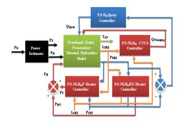
**Fig. 1.** Proposed closed loop pressurizer pressure and level control system.
