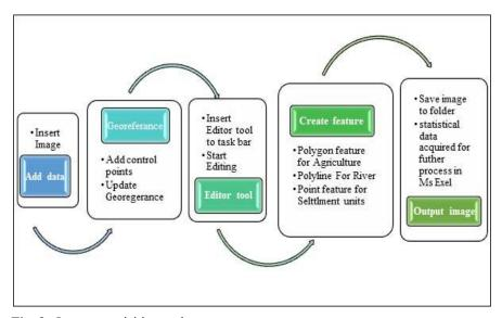
Fig. 3. Image acquisition and process
