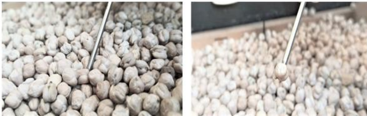
Fig. 3. Recording temperature and seed moisture at different depths using pointed sensor needle [21]
