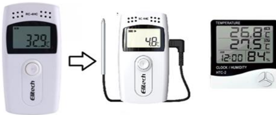
Fig. 2. Data logger and digital thermometer for recording temperature and Humidity [21]
