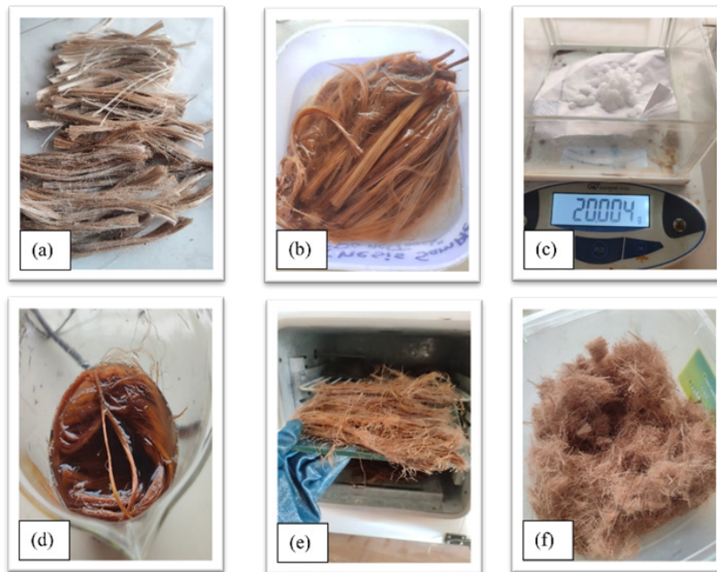
Fig. 2. Jute fiber treatment, (a) Jute fiber cut into 6 inches, (b) Washing jute, (c) Weighing NaOH, (d) Jute soaked in NaOH, (e) Drying in oven, and (f) Cut into 10mm.
